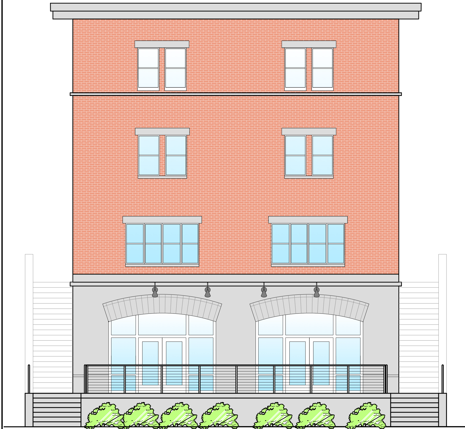
CHURCH STREET ELEVATION EXPANDED DECK - NEW RAILING
