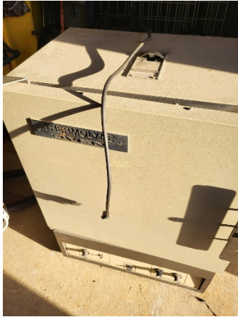
WWTP – drying oven
