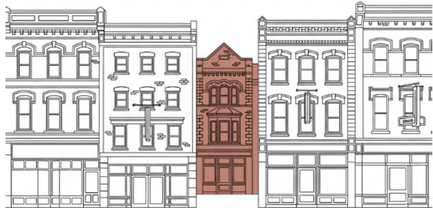
Inappropriate setback of infill construction.
