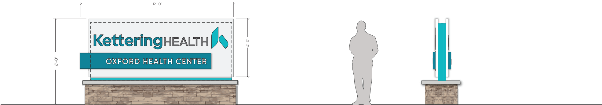
Sign Elevation: Ground Monument 1 Scale: 3/8" = 1'-0" 8.00
