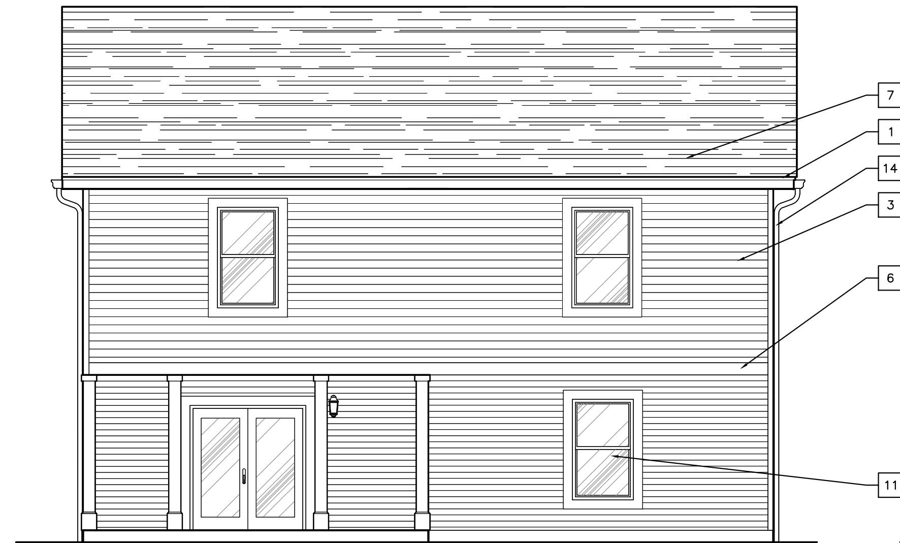
2 DUPLEX BUILDING D2 REAR ELEVATION B1 SCALE: 3/16"=1'-0"
