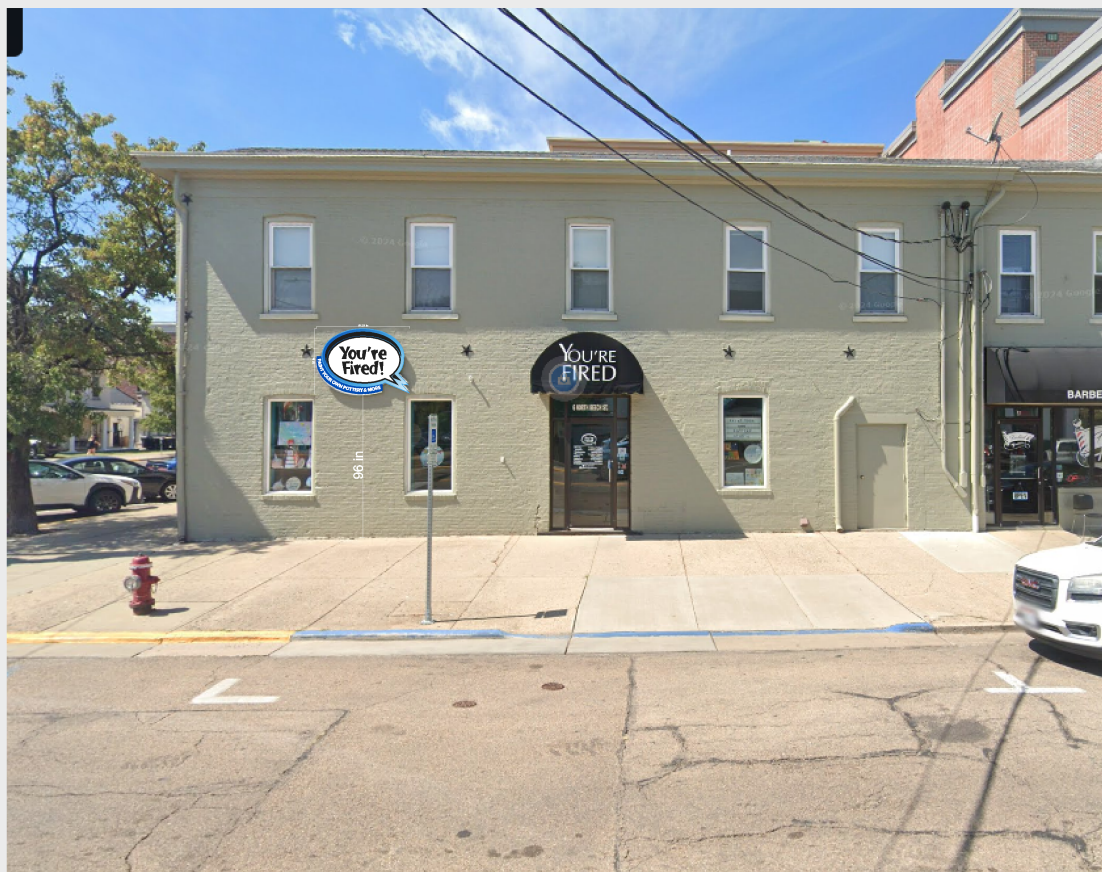
6mm laminated aluminum cut out sign wall mounted with 6 - 2.25" lag screws
